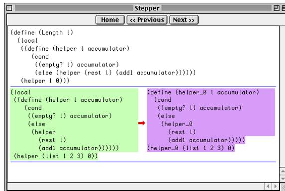
Figure 7. Reducing `local` (MacOS version).
