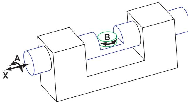
Figure 2: Our rotary-linear (A-X) axis eliminates the conventional stacking of axes.
