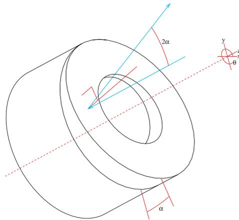
Figure 4: Plane mirror interferometry off a tilted mirror maps rotation into displacement. The angle  $\alpha$  is limited by the angular acceptance of the light detector.
