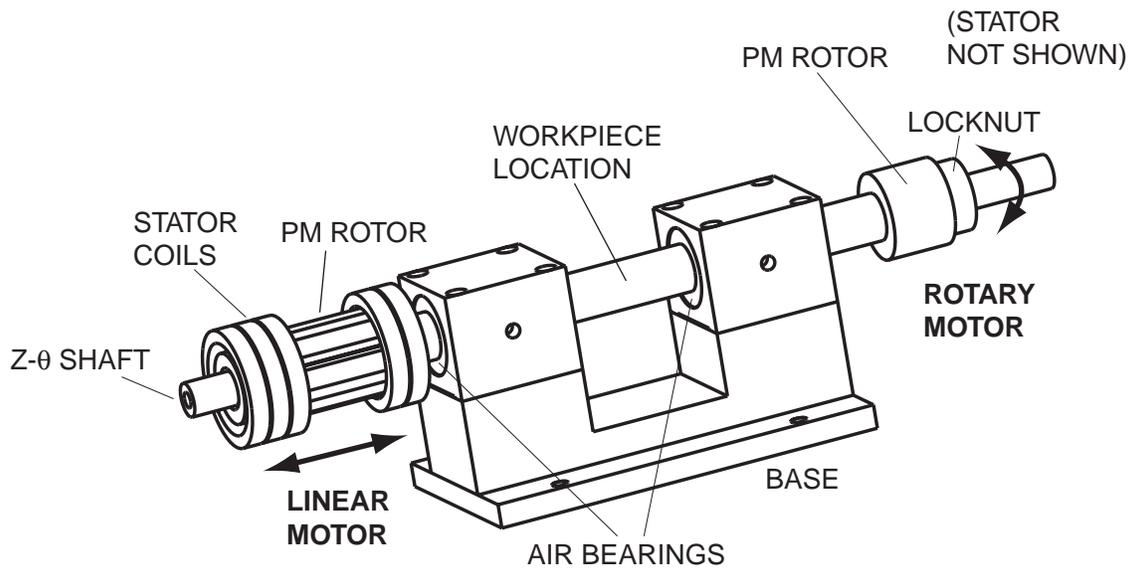
Figure 3: A rotary-linear hybrid axis. The central shaft is mounted in air bearings and has permanent magnet rotors for linear and rotary motors attached to it.
