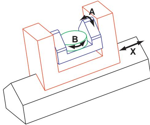
Figure 1: A common stacked-axis arrangement used in horizontal multi-axis machine tools. A rotary index table (B) is mounted on a trunion (A) which is moved by a linear axis (X).
