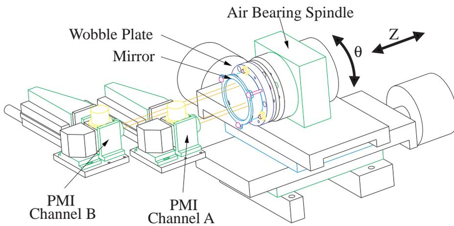
Figure 5: Experimental setup for testing the tilted mirror sensor.
